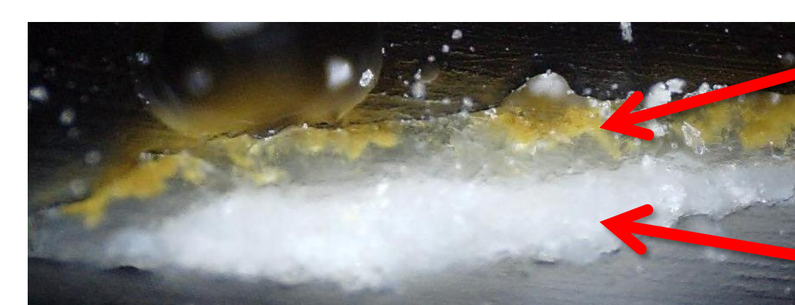
Olive brown glaze in cross-section 100X with polarized light microscope, visible light
