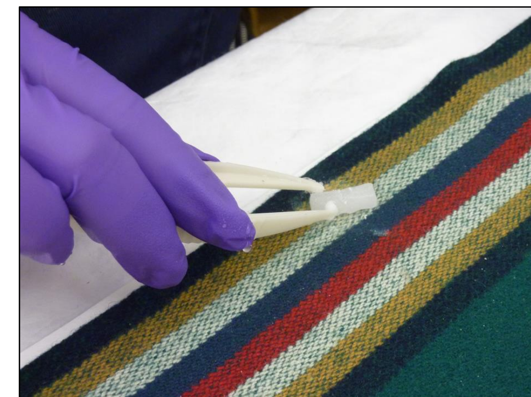
Applying dry ice directly to an accretion, as in step 5.
