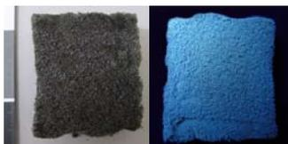
Figure 11: Foam squares cut to 3x3 inches approximately were prepared for consolidation experiments and were photographed in visible and UV light before and after consolidation experiments.
