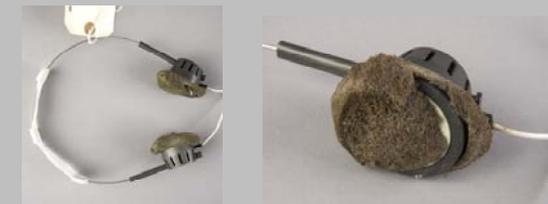
Figure 2 and 3: Details of the headset and the foam ear-cushions before treatment condition: The most significant area of deterioration on the headset is the polyurethane (PUR) ester foam ear-cushions which are stiff, brittle, and actively crumbling to powder. There are deformations, indentations, and cracks. Additionally, the foam has no characteristic spring-back.
