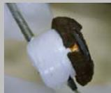
Figure 5: Plastic component wrapped with Teflon tape before treating the foam.
