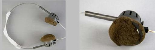
Figure 6 and 7: (Left) overall, (right) detail of PL ear-cushion: The ear-cushions are now structurally stabilized as evidenced by the lack of shedding foam. The hardness of the foam is still present, however, the brittleness has subsided and slight spring-back is observed. The color appears as a deep brown tone, which is different from its before treatment gray-brown color.
