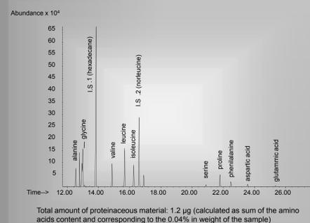
**Figure 5.** Gas Chromatographic Mass Spectrometric analysis: Single Ion Monitoring (SIM) of the amino acid fraction.
