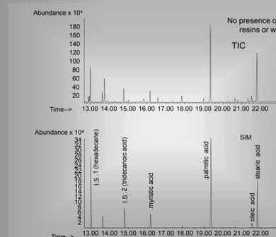
**Figure 7.** Gas Chromatographic Mass Spectrometric analysis: Total Ion Chromatogram (TIC) and Single Ion Monitoring (SIM) of the lipid resinous fraction.
