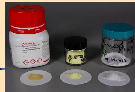
Figure 5: Color comparison between original phenylene bismaleimide (left), purified phenylene bismaleimide (center), and hexylene bismaleimide (right)
