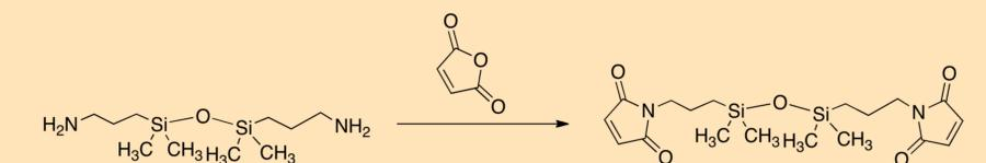
Figure 8: Schematic for siloxane bridged bismaleimide
