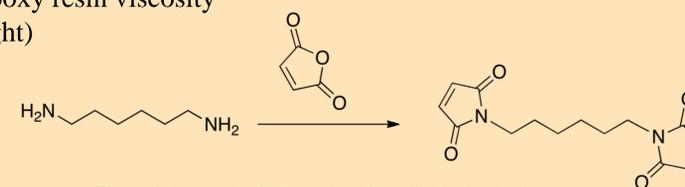
Figure 6: Schematic of 1,6-hexylenebismaleimide chemical structure
