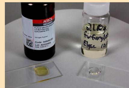
Figure 5: Original and purified furfuryl glycidyl ether
