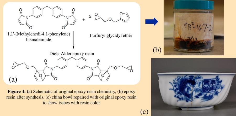
Figure 4: (a) Schematic of original epoxy resin chemistry, (b) epoxy resin after synthesis, (c) china bowl repaired with original epoxy resin to show issues with resin color
