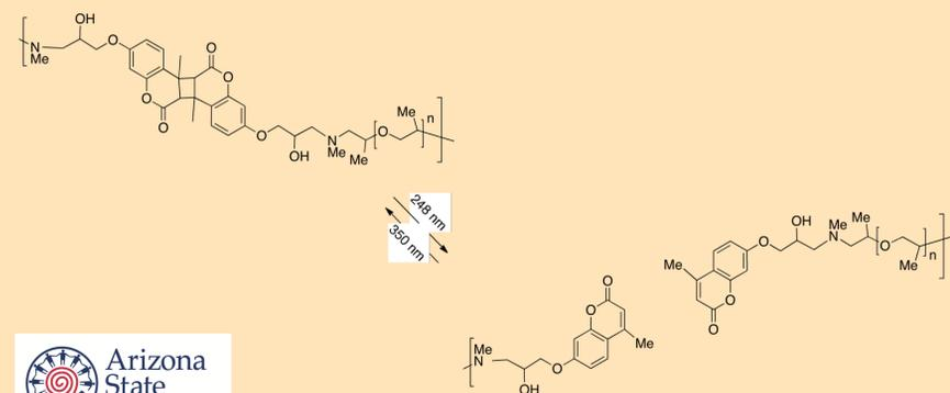
Figure 3: Coumarin dimer reaction incorporated into epoxy. Epoxy is solid at wavelengths above 300 nm and liquid at wavelengths below 300 nm
