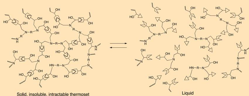
Figure 1: Schematic of solid epoxy structure with weak links intact and liquid epoxy structure with weak links detached
