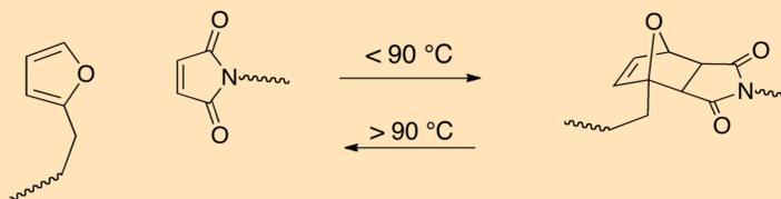
Figure 2: Diels-Alder reaction incorporated into epoxy. Epoxy is solid at temperatures below 90 °C and liquid above 90 °C
