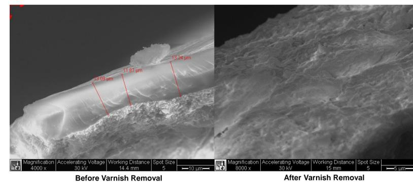
**Figure 6.** ESEM images before and after varnish removal. Note, ESEM imaging required removal of a small (approximately 1 mm<sup>2</sup>) portion of the painting. Measured varnish layer thickness in three locations: 13.09  $\mu\text{m}$ , 11.87  $\mu\text{m}$  and 13.24  $\mu\text{m}$ . In the image acquire after Er:YAG removal, the surface of the paint appears devoid of varnish, and the texture of the surface of the painting appears fluid-like with pockets of smoothed areas.
