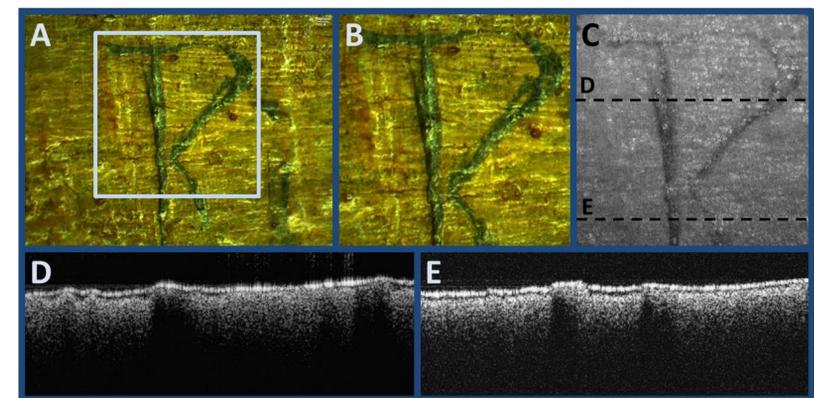
**Figure 5.** Images of the signature on an oil on wood 19<sup>th</sup> century Venetian landscape painting by Rico. Microscope image of the R in the signature acquired at 4x magnification (A), close-up of A indicated by the light blue box (B), OCT SVP of the same region shown in B (C), OCT cross-sectional images (D & E) acquired along the dotted lines shown in C.
