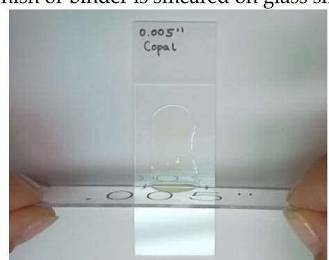
A thickness of 5mills is achieved using a coverslip Slide is placed on a hot plate (80°C) for artificial
