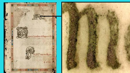
Figure 6 – Detail of metallic pigment degradation. The green coloration indicates the use of brass instead of gold to illuminate the letters.
