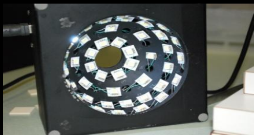
The underside of the Monkey Brain. The programmed software automatically snaps a photo as each LED lights up in sequence.
