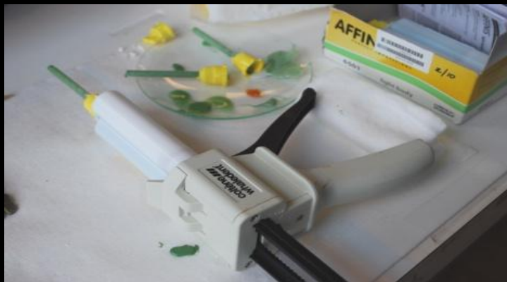
Polysiloxane impression material by Affinis, Coltene Light Body 6501, used for taking impressions and the impressions seen above.
