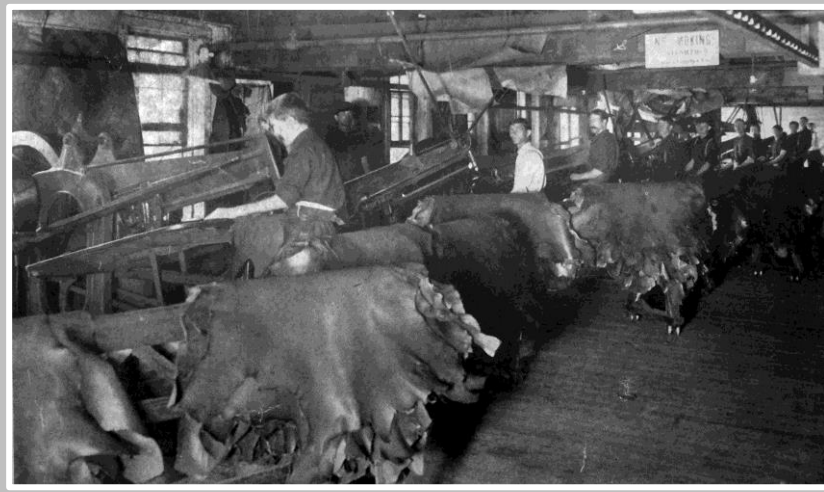
Staking Chrome Tanned Calfskin in a Shoe Upper Leather Tannery – Philadelphia, 1910 (Flemming, L. A. 1910. Practical Tanning: A Handbook of Modern Processes , Philadelphia: Henry Carey Baird & Co.)
