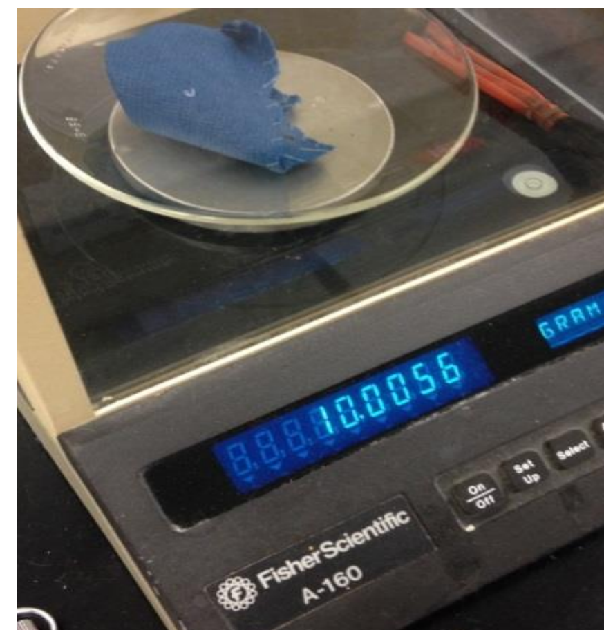
Wet sample re-weighed to determine amount of water absorbed
