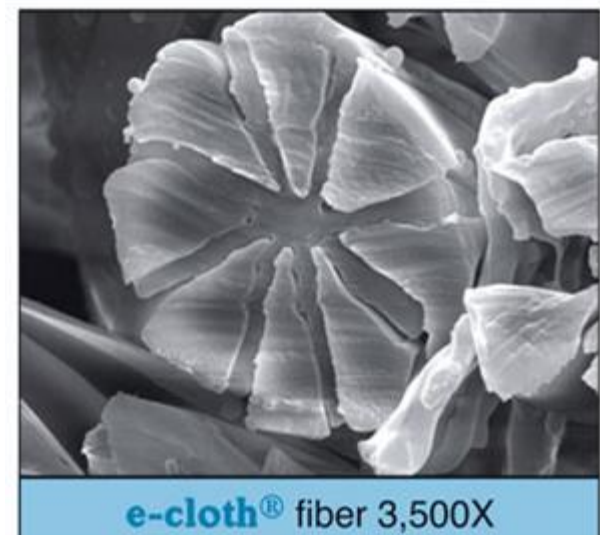
(Cross-sectional view of bi-component, Star-shaped microfiber. Photo courtesy of E-cloth, accessed from website March 28, 2016)
