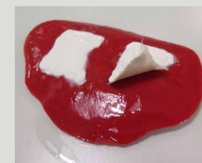
7. Testing the reversibility in water of Modostuc over Japanese paper and isinglass on wax after a 48 hour drying time.
