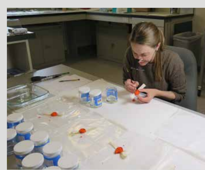
1. Testing water-soluble consolidants in a variety of strengths including isinglass, JunFunori, and Aquazol 50, 200, and 500.
