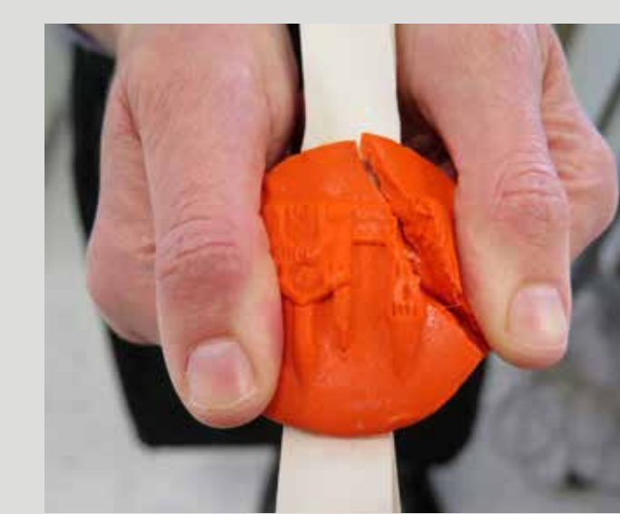
3. Low-tech tensile strength testing. Isinglass appeared much stronger than Aquazol after a 48 hour drying time.
