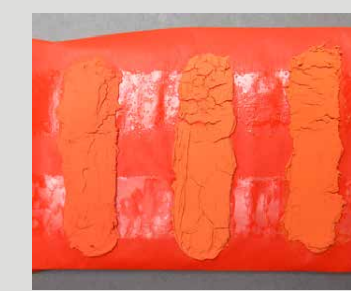
4. Pigmented fill material over Aquazol (upper horizontal band) and isinglass (lower horizontal band) on wax. The Aquazol beaded up on the wax surface, but the isinglass did not. Modostuc (left) was more stable than Flügger or Aquazol-based fill materials.
