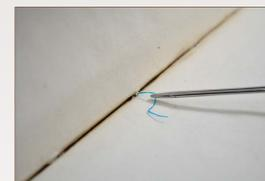
Using the alligator forceps to grasp the beading wire in the space between the textblock and the spine of the cover.
