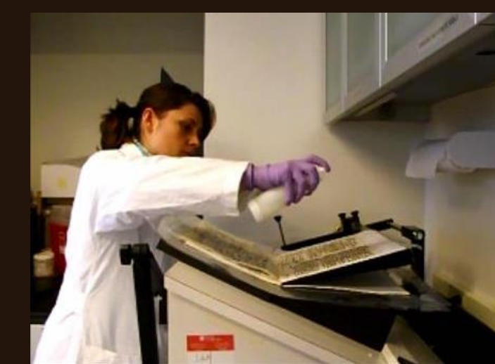
Application of Bookkeeper® on the book suction machine during the tests
