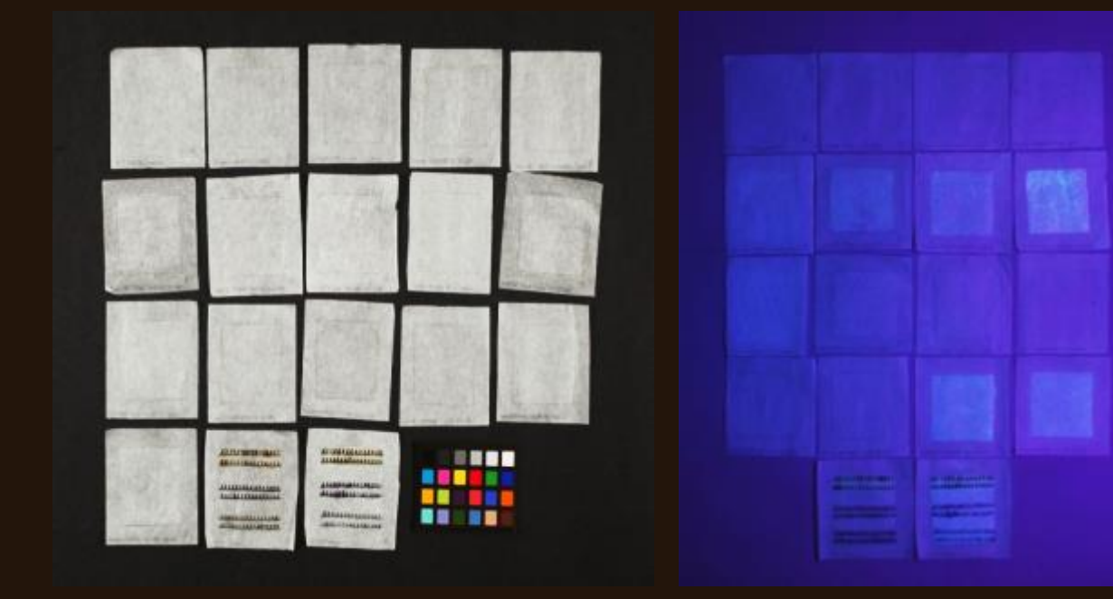
Adhesives on squares of Silk Natural paper after aging
