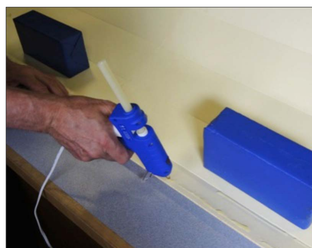
After folding, the small flap is hot-glued. We found that a slow-set glue, rated at 45-seconds, was needed.
