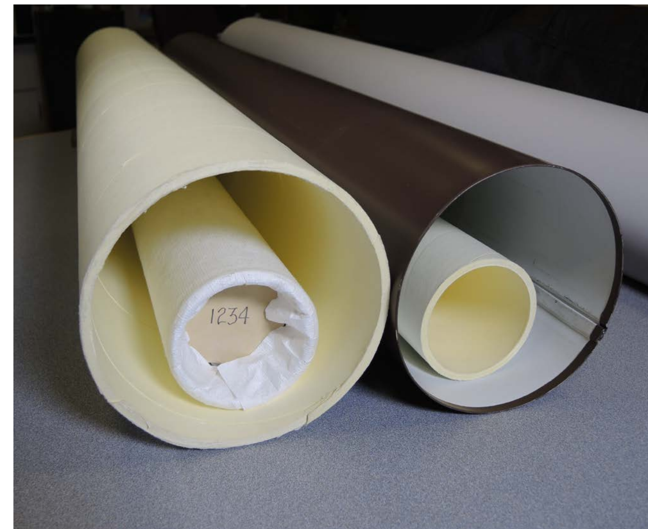
Early considerations for storage included the 6" acid-free tube; a custom-made aluminum tube, and a box fabricated from Coroplast. In this photo the Coroplast is supporting 36 lbs. of weight.
