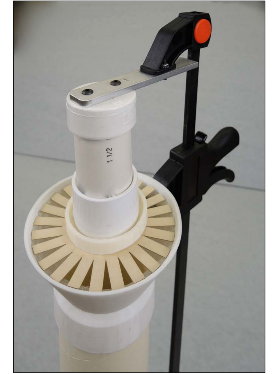
This funnel-shaped device and the plunger were 3-D printed using Library facilities. The device is used to insert the label into the tube.
