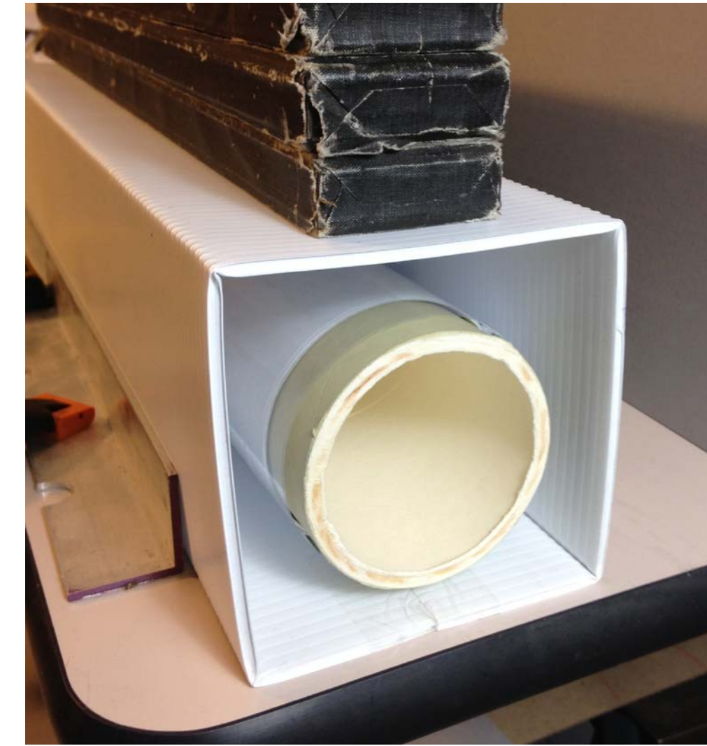
Early considerations for storage included the 6" acid-free tube; a custom-made aluminum tube, and a box fabricated from Coroplast. In this photo the Coroplast is supporting 36 lbs. of weight.
