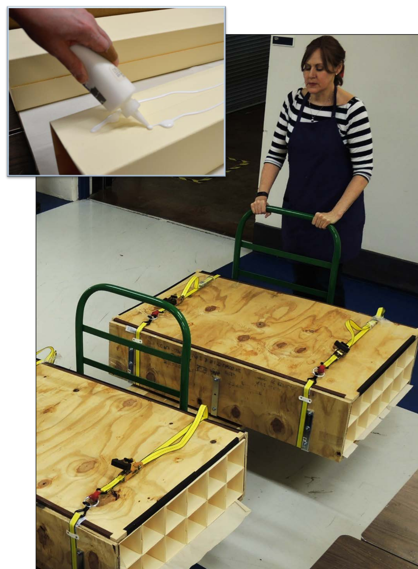
Individual boxes were then assembled into twelve-box units using PVA. They were then placed in these wooden frames for 20-minutes while the PVA set.
