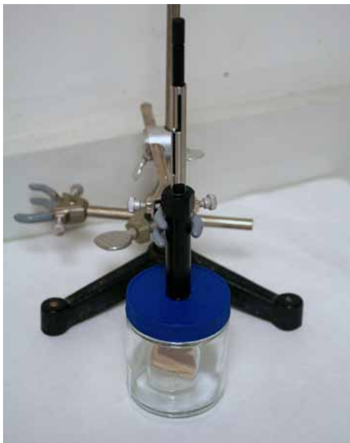
Fig. 1b: SPME fiber exposed in a modified MMA Oddy test vessel. Photographs by Masahiko Tsukada. Images © The Metropolitan Museum of Art.
