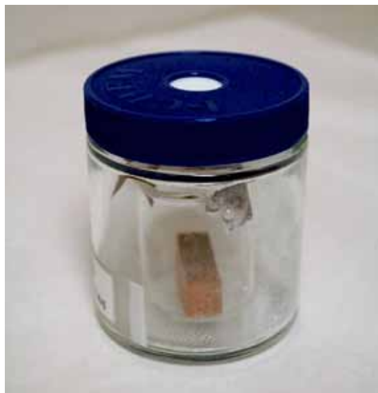
Fig. 1a: Modified MMA Oddy test vessel with septum;
