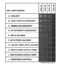
ISO blue wool test samples show almost no fading with NoUVIR even after 250,000 footcandle/hours (roughly 10-exhibit years) of light exposure.
