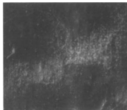
Figure 10. Photomicrograph ( \times 500 ) of UC14692 (Figure 1) showing hazy bloom (photo: Libby Sheldon/Noëlle Streeton)
