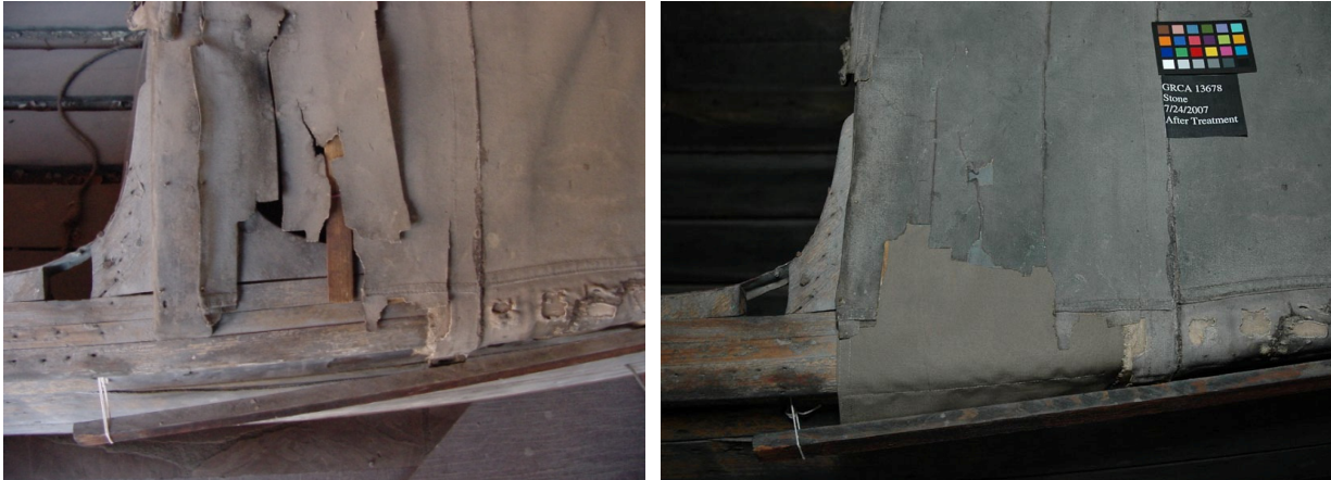
Fig. 6. Before (left) and after (right) treatment of the canvas deck on the Stone boat (Photographs by Brynn Bender)
