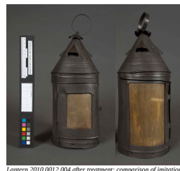
Lantern 2010.0012.004 after treatment: comparison of imitation (right) and original (left) panes.
