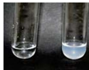
Figure 5: Chloride ion test with silver nitrate solution, showing a negative reaction with the distilled water control (left) and a positive reaction with the shard soaking bath (right).
