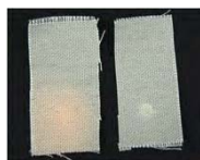
Figure 4: Spot tests with concentrated hydrochloric acid (left) and hydrogen peroxide (right) applied directly to unwashed display case fabric.
