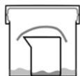
Figure 7: Experimental set-up for indirect exposure of fabric strips to hydrochloric acid or hydrogen peroxide cleaning solutions.
