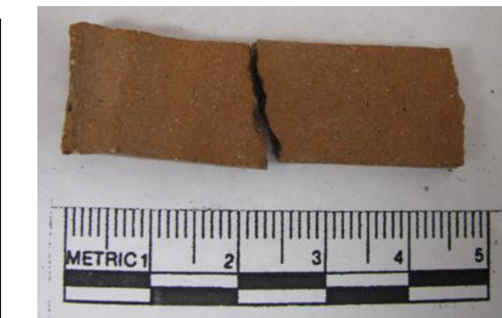
Gila plain sample after 1 month of accelerated aging (left) and after two months (right). The only noticeable difference is the presence of a white efflorescence on the surface after two months. No damage or crumbling of the surface visible.
