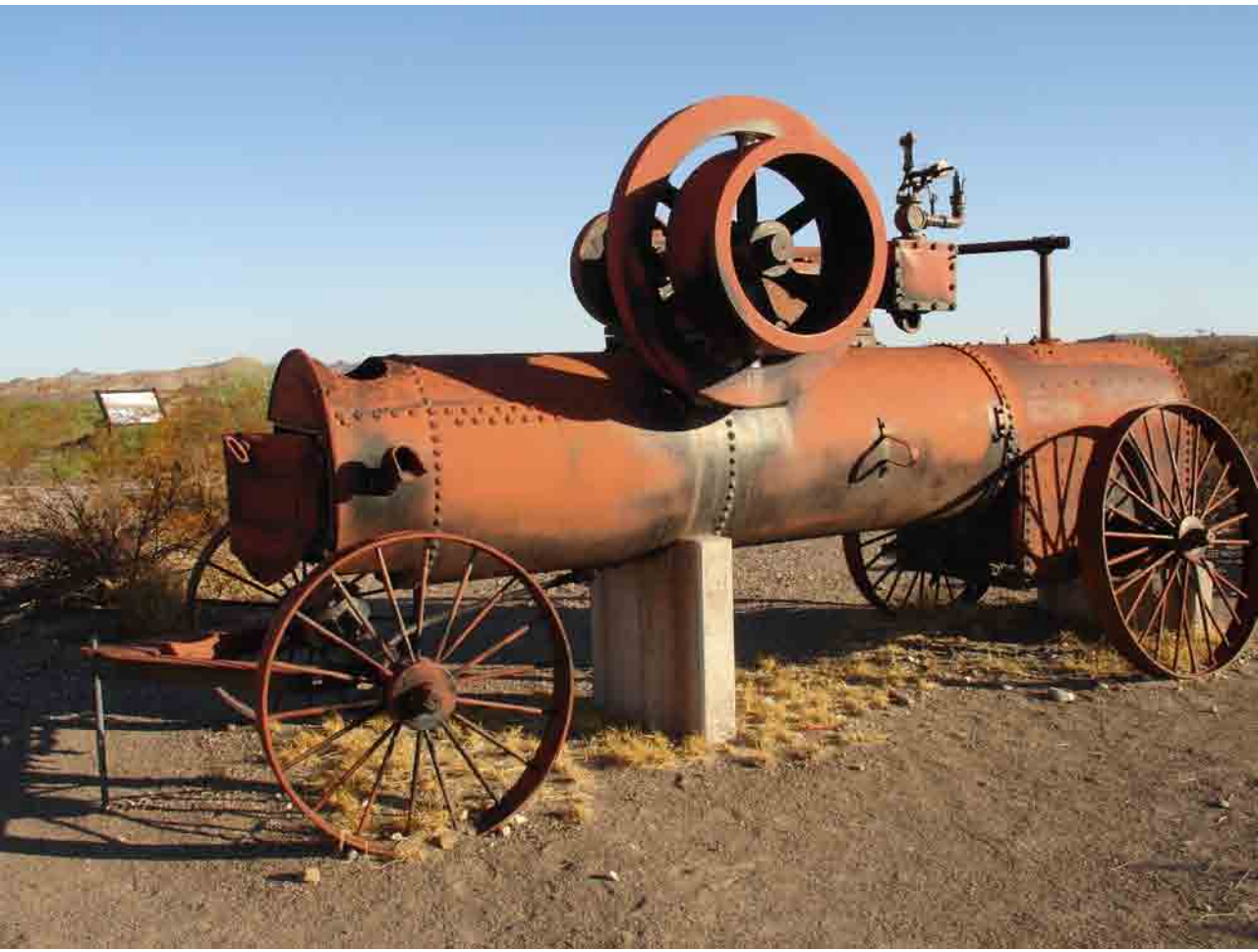
Steam Engine at Big Bend National Park in Texas. Much of the original coating and some of the primer has been worn away by wind blowing sand. Photo by Dana K. Senge
