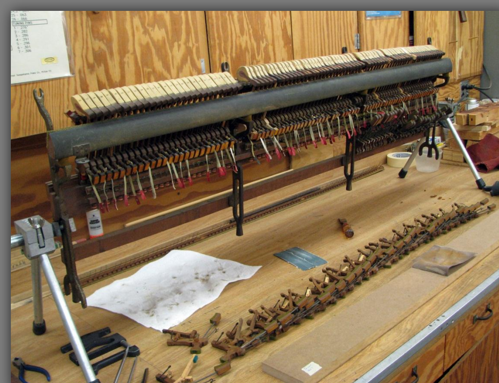
The hammer mechanism during treatment. Worn hammer shanks and felt pads were replaced.
