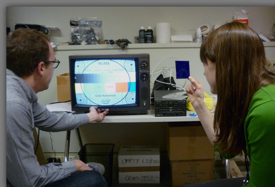
Peter Oleksik and Emily Hamilton calibrate a monitor using a blue gel filter. When looking through the filter, it is possible to tell when the colors are balanced.
