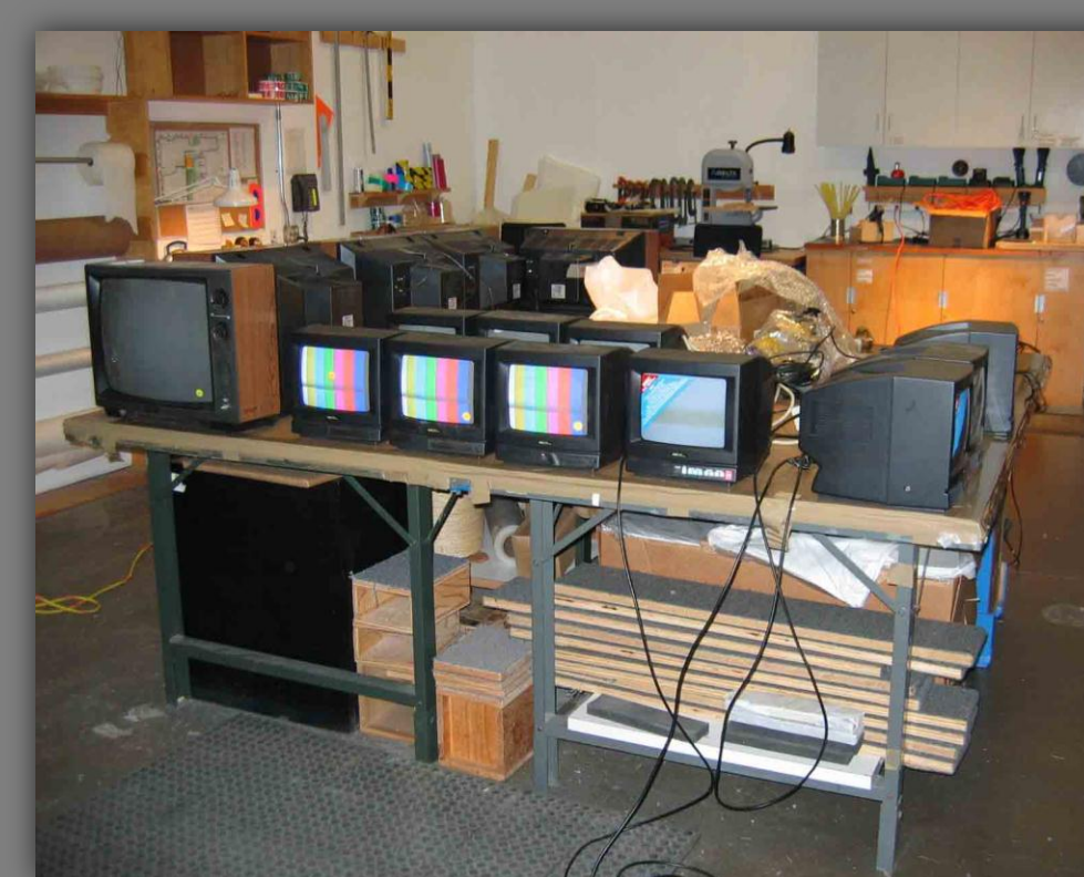
The CRT monitors were tested and calibrated as a group at MoMA.
