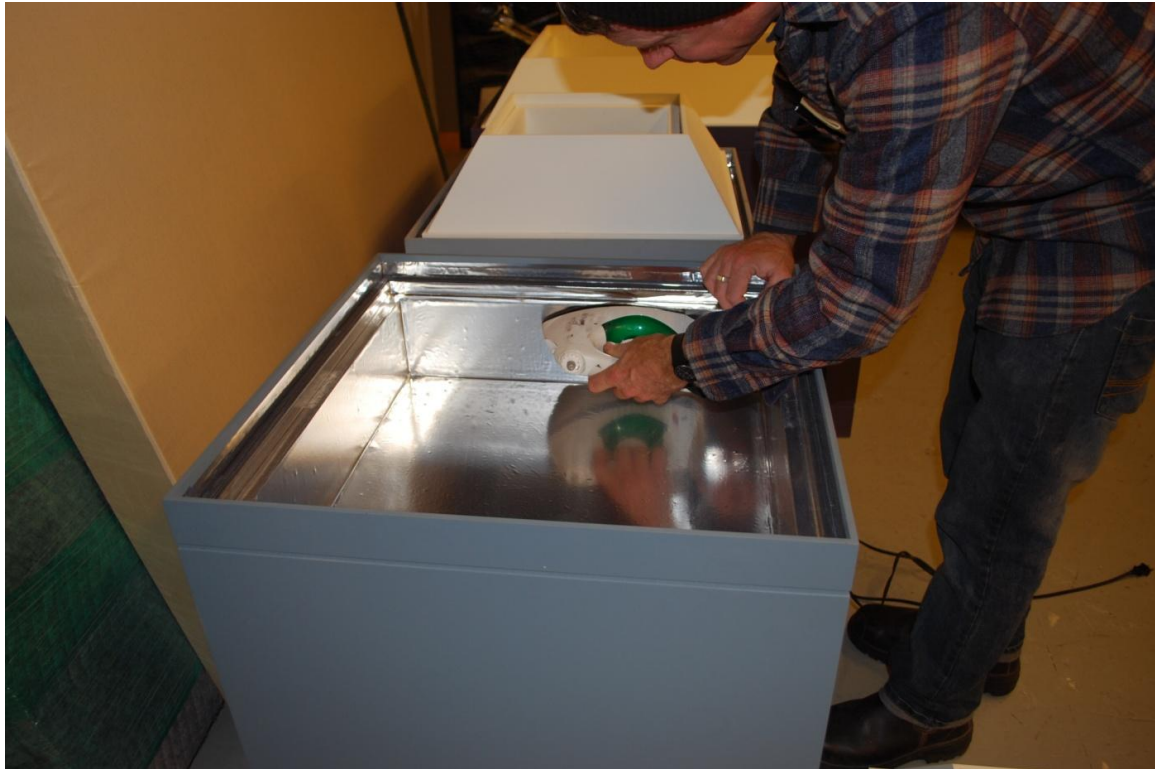
IMLS supported Exhibition Technician Michael Bouyacas using a conventional iron to apply Marvelseal 360 to the silica gel sub compartment.
