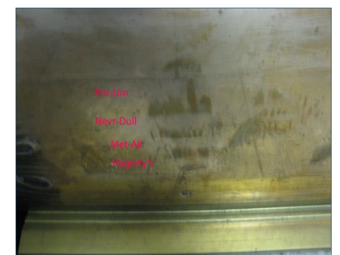
Polishing tests on reproduction brass door hardware
