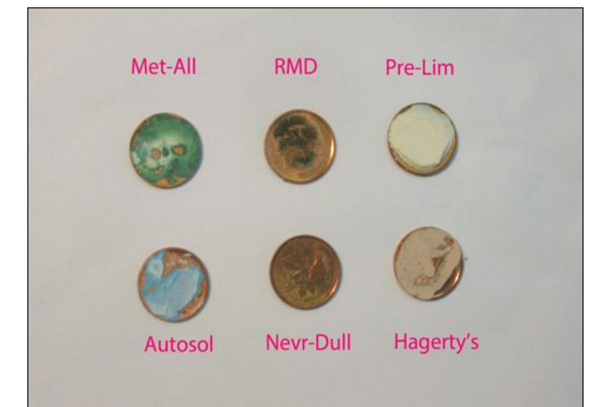
Polish residues on pennies (copper alloy) after 24 hours – a persuasive visual aid
