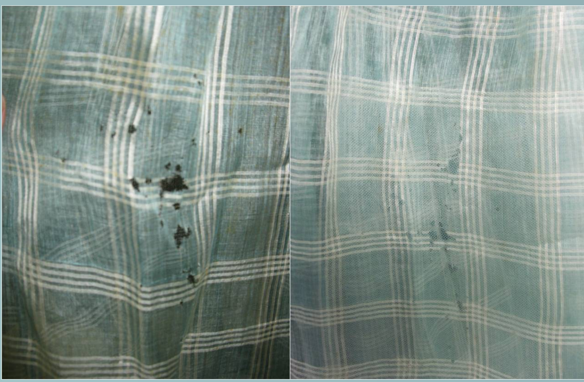
Insect damage to silk taffeta before conservation (L) and after stabilization with silk crepe line (R).
