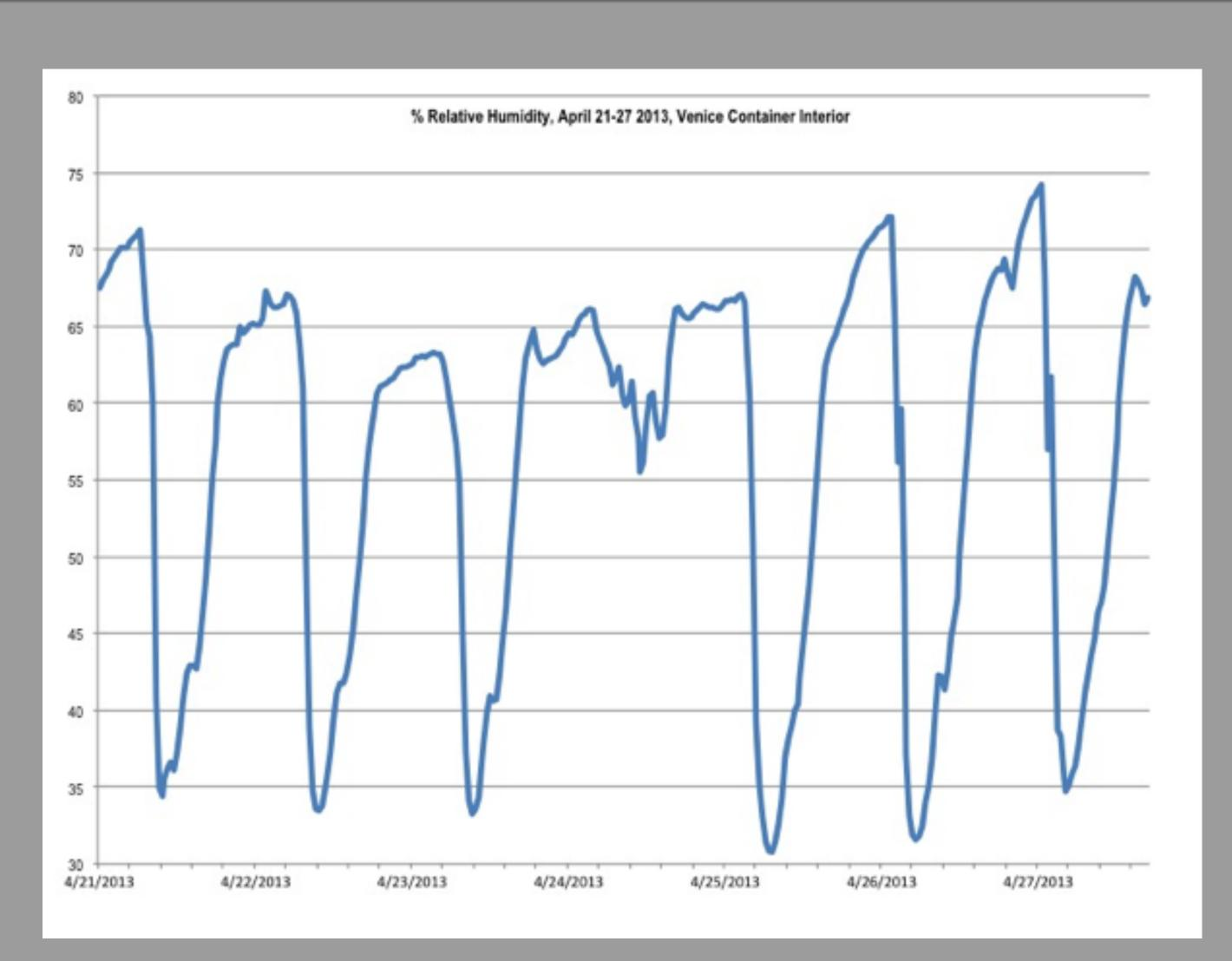
The percent relative humidity fluctuated by up to 56.5 percent during the course of each day inside the Venice container. On April 24<sup>th</sup> the percent relative humidity never dropped below 55 percent, illustrating a discrepancy likely caused by container use or a weather event.
