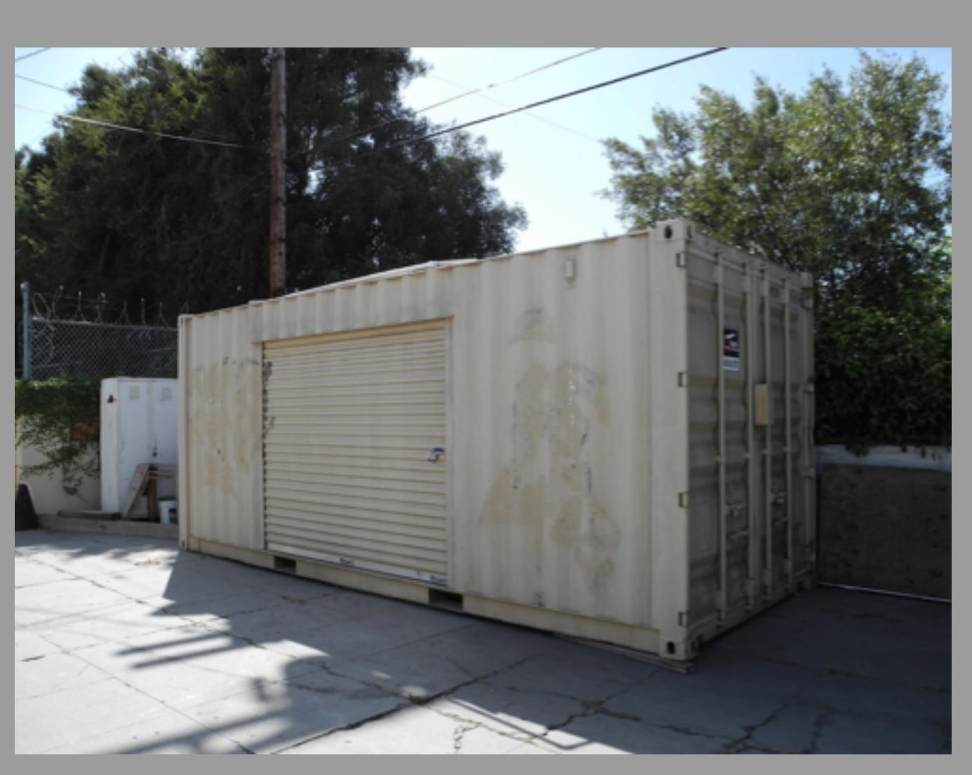
The Venice container is an uninsulated, single-walled 20-foot ISO standard shipping container, positioned directly on concrete. It is painted tan, relies solely on natural ventilation, and is not outfitted with a canopy or covering.
