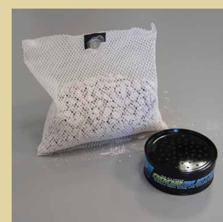
Attempts were made to reduce the musty odor of the fans. Fans were placed into an ArtCare storage box within a fume hood. Inside the box, the fans rested on a MicroChamber paper sling above odor-absorbing materials. Activated carbon (Tub O'Carbon) proved to be less messy and was chosen over zeolites (Gonzo Odor Eliminator).
