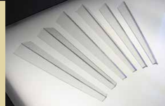
Vivak 099 forms were used as supports to facilitate mending while working over a light table.
