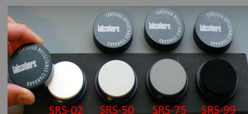
Figure 4: A set of Spectralon Diffuse Reflectance Standards was included in each image. The spectral responses for these standards (SRS-02, SRS-50, SRS-75, SRS-99) between 350 nm to 1100 nm are highlighted by the red box to the left.
