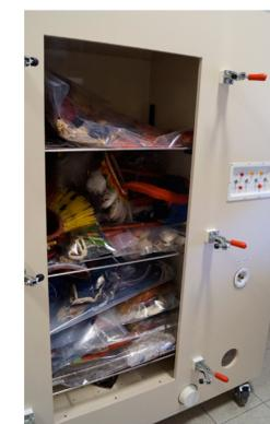
Portable nitrogen fumigation chamber
