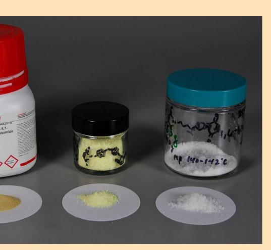
Figure 5: Color comparison between original phenylene bismaleimide (left), purified phenylene bismaleimide (center), and hexylene bismaleimide (right)
