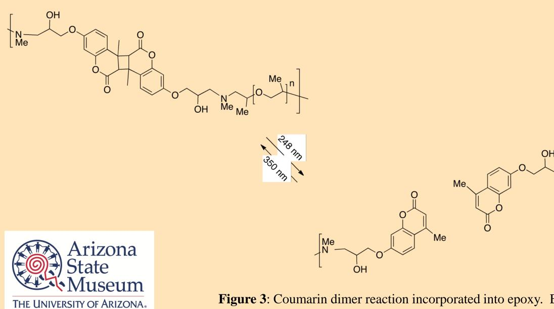
Figure 3: Coumarin dimer reaction incorporated into epoxy. Epoxy is solid at wavelengths above 300 nm and liquid at wavelengths below 300 nm
