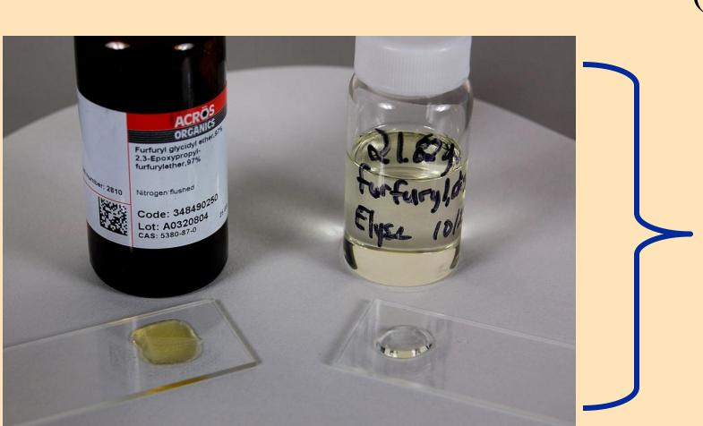
Figure 5: Original and purified furfuryl glycidyl ether
