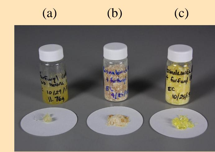
Figure 7: Epoxies synthesized from purified and unpurified components.
