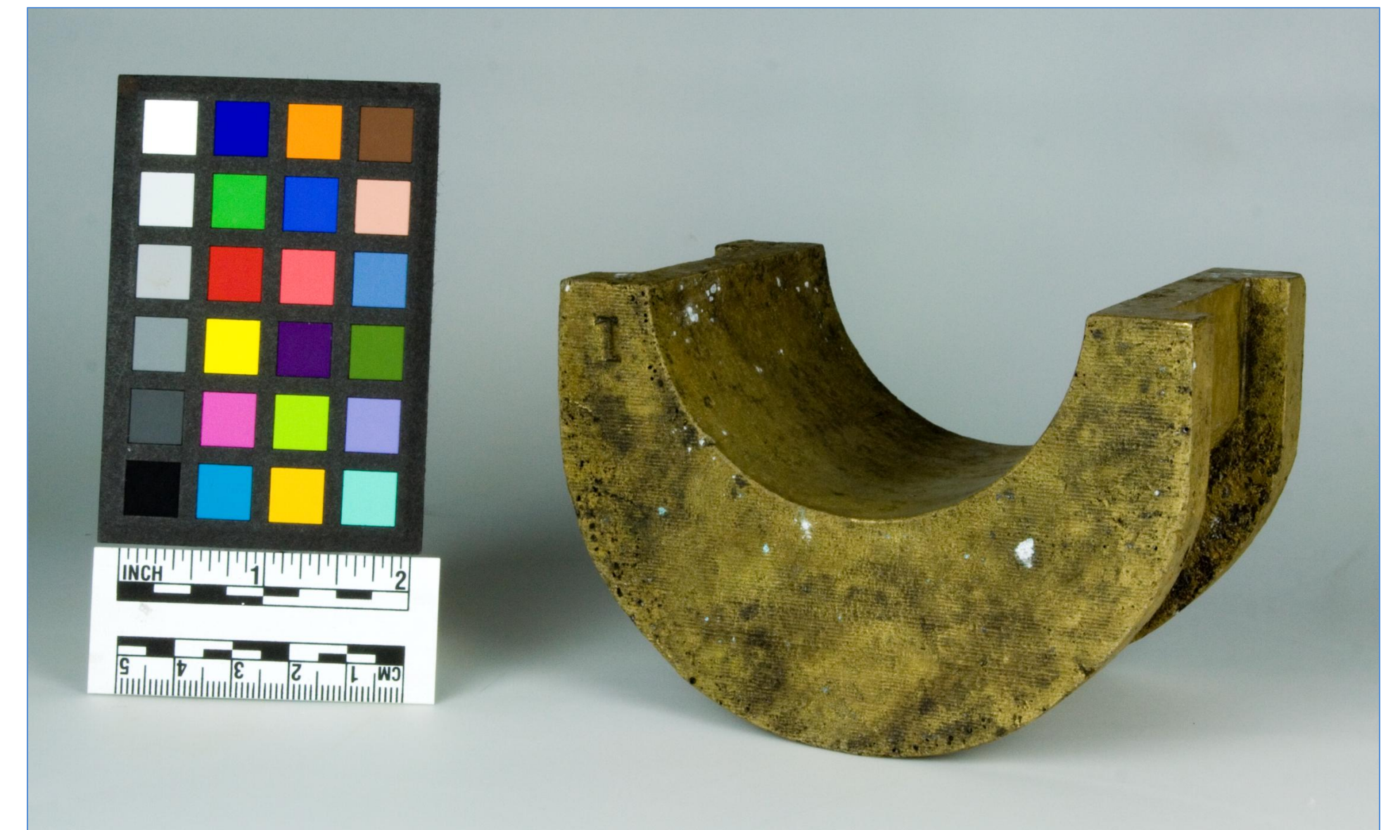
Figure 4: Artifact MNMS.2001.003.219, a copper alloy bearing before retreatment. The white powdery bloom is visible on both the exterior and interior surfaces. Image courtesy of The Mariners' Museum
