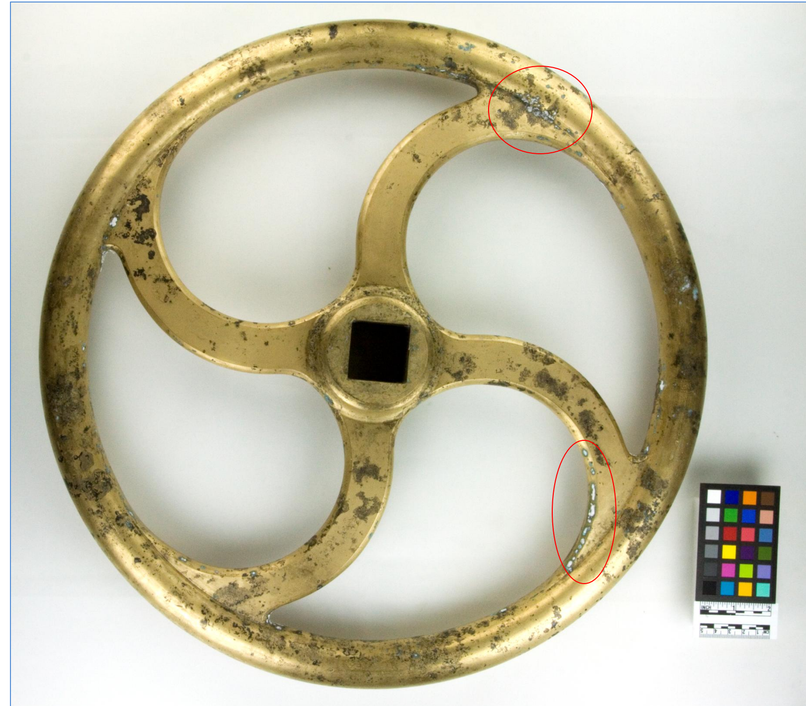
Figure 3: Artifact MNMS.2002.001.469B1, a copper alloy wheel before retreatment. The largest areas of white bloom are indicated with a red circle. Image courtesy of The Mariners' Museum.
