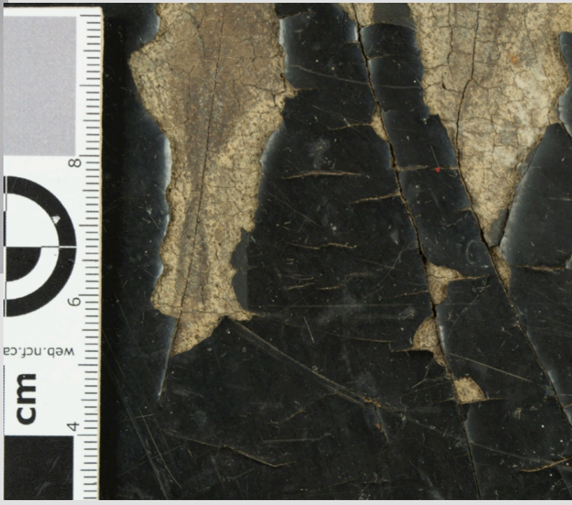
Fig 6: Marubon BT, flaking lacquer underside
