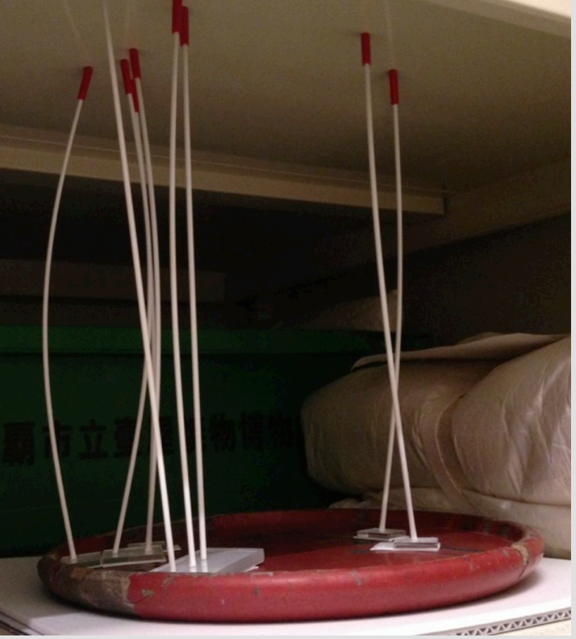
Fig 7: Japanese shimbari clamping method
