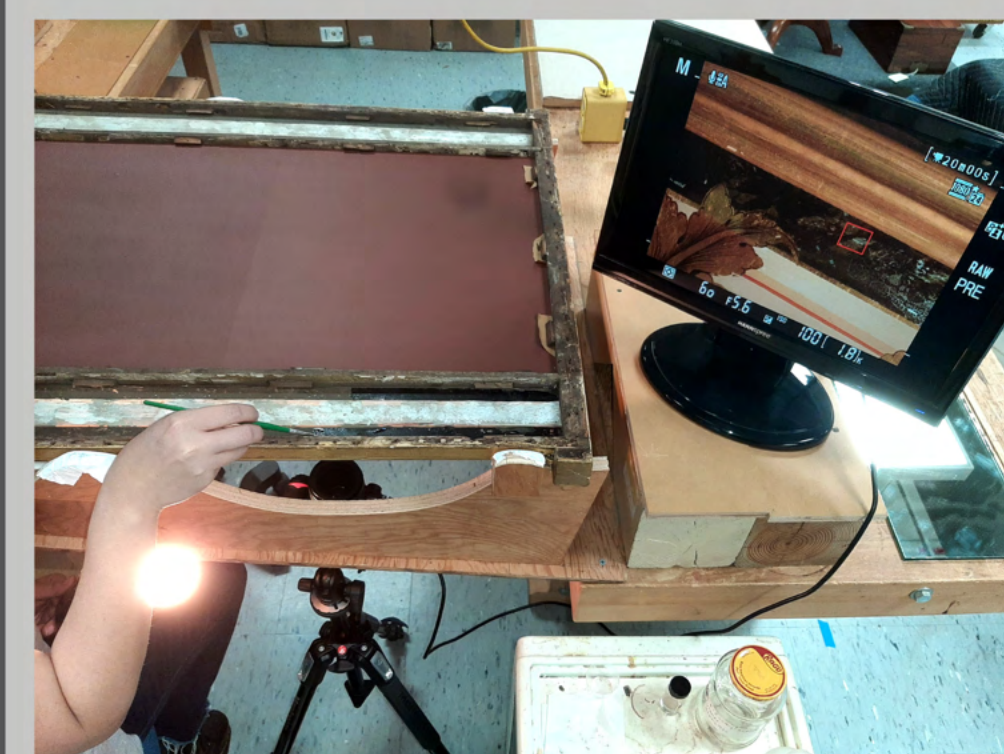
Camera on tripod placed below mirror. Set to "live feed" view, hooked up to a computer monitor
