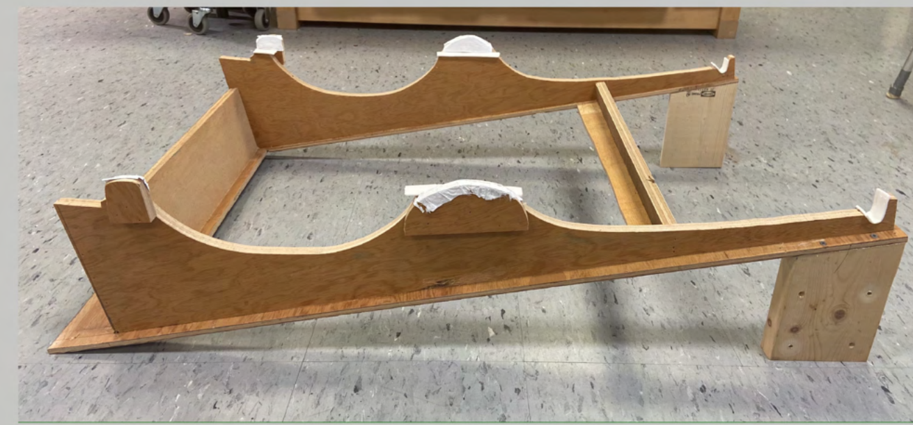
Custom mount designed to hold the mirror horizontally, rear side up
