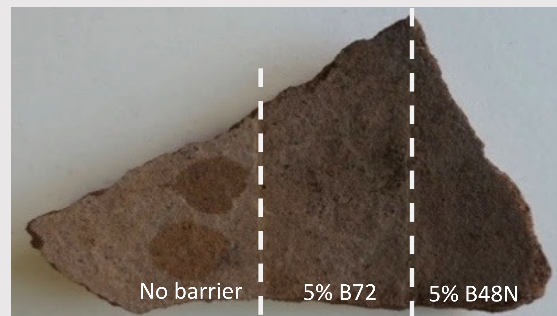
Figure 1. Earthenware sherd with two spots of siloxane staining (left third) and darkening from B72 & B48N barriers, after attempted removal with solvent.
