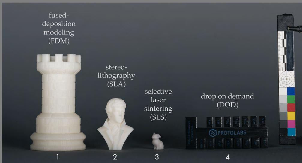
Figure 1: 3D printed samples photographed in normal light (N).
