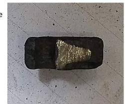
Figure 9: A sample which has been cut rather than broken, showing the extent of core metal remaining.
