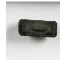
Figure 8: A sample from the full-scale generation, broken in half to show the structure. The exterior is fully graphitized. Below this is an iron-depleted layer which is no longer metallic, but is substantially harder and denser than the outer layer. At the center is a core of metallic cast iron.
