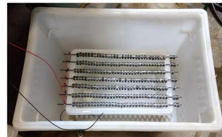
Figure 7 (Below) Samples undergoing electrolytic corrosion.
