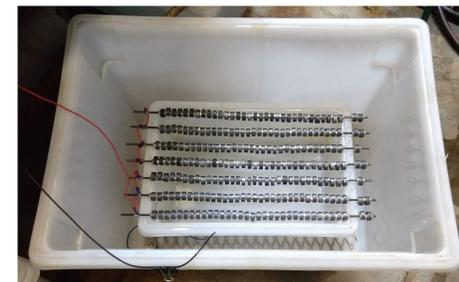
Figure 7 (Below) Samples undergoing electrolytic corrosion.
