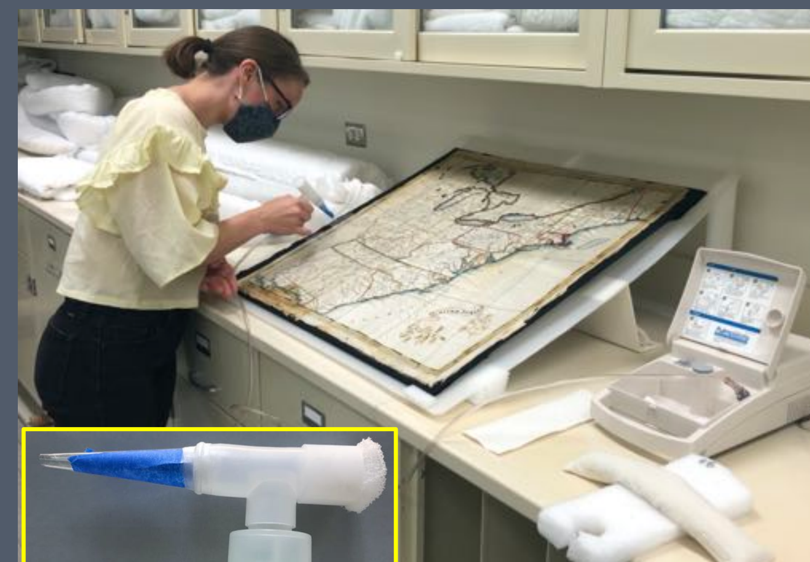
Fig. 5. Mist consolidation treatment in action. Sampler placed on a mount at a 30-degree angle. Inset image: Pulmomate nebulizer modified with a Mylar to create a fine nozzle.
