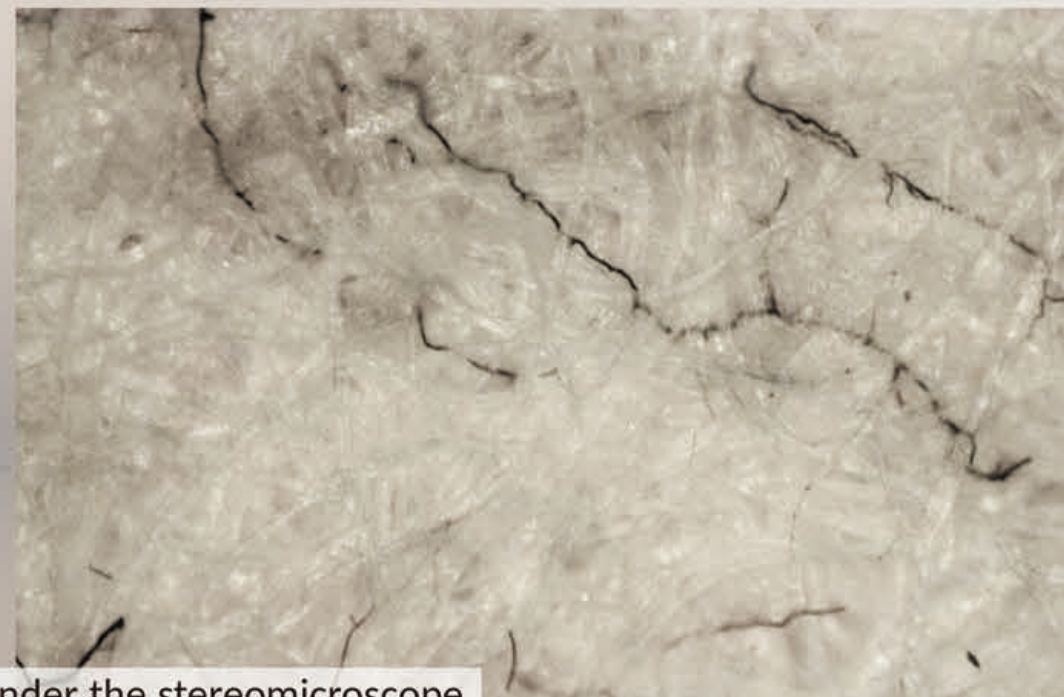
Fig. 7 The 500X image under the stereomicroscope shows that the relationship between paper fibers and mold is just like earth and plant roots.
