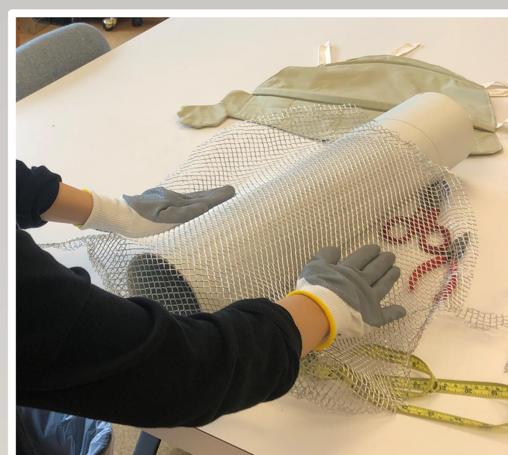
Fig 4. Initial shaping of the Formetal® using tin snips and an archival tube.
