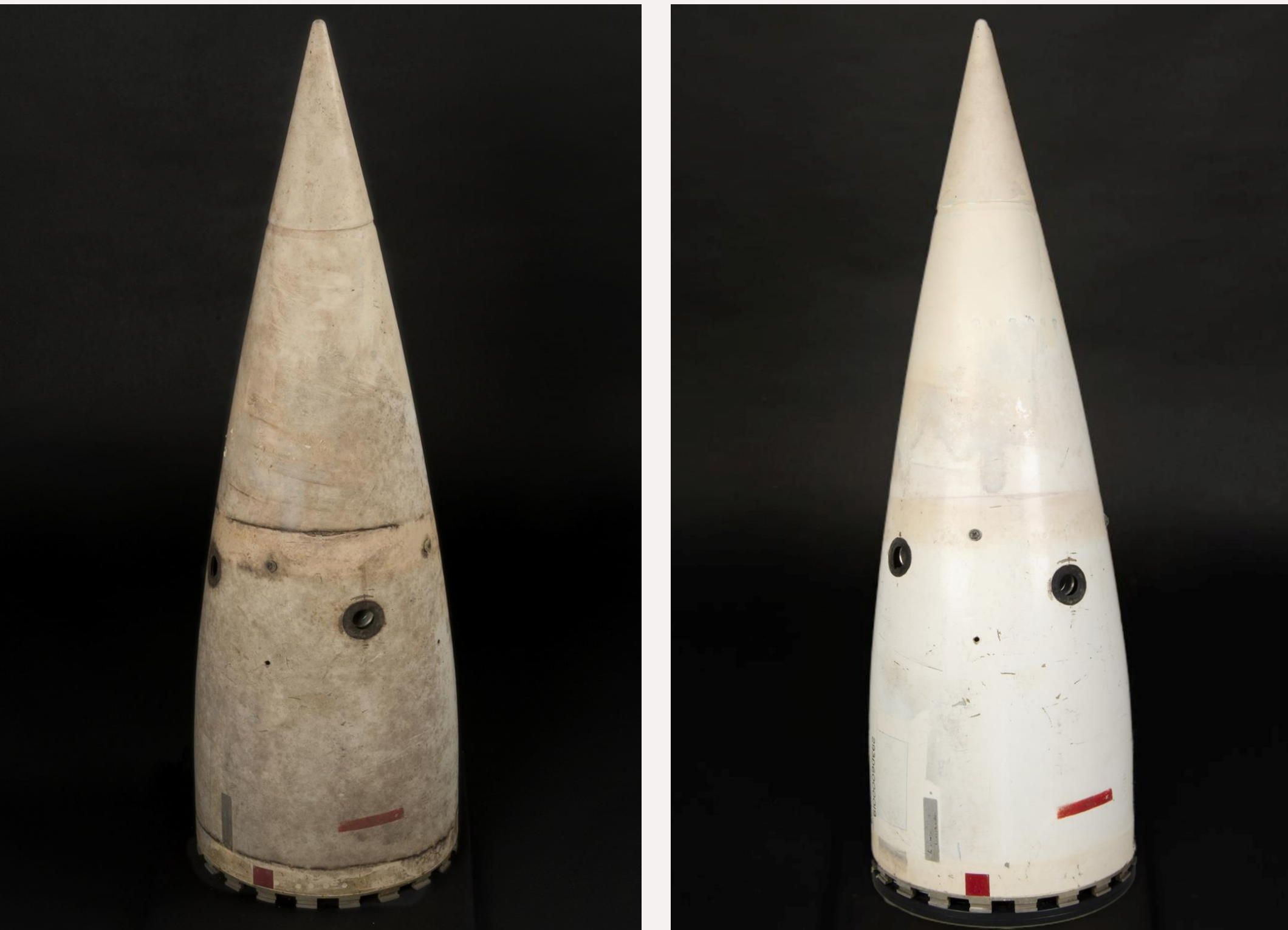
BT, nose cone (left). AT, following oxalic acid (right).
