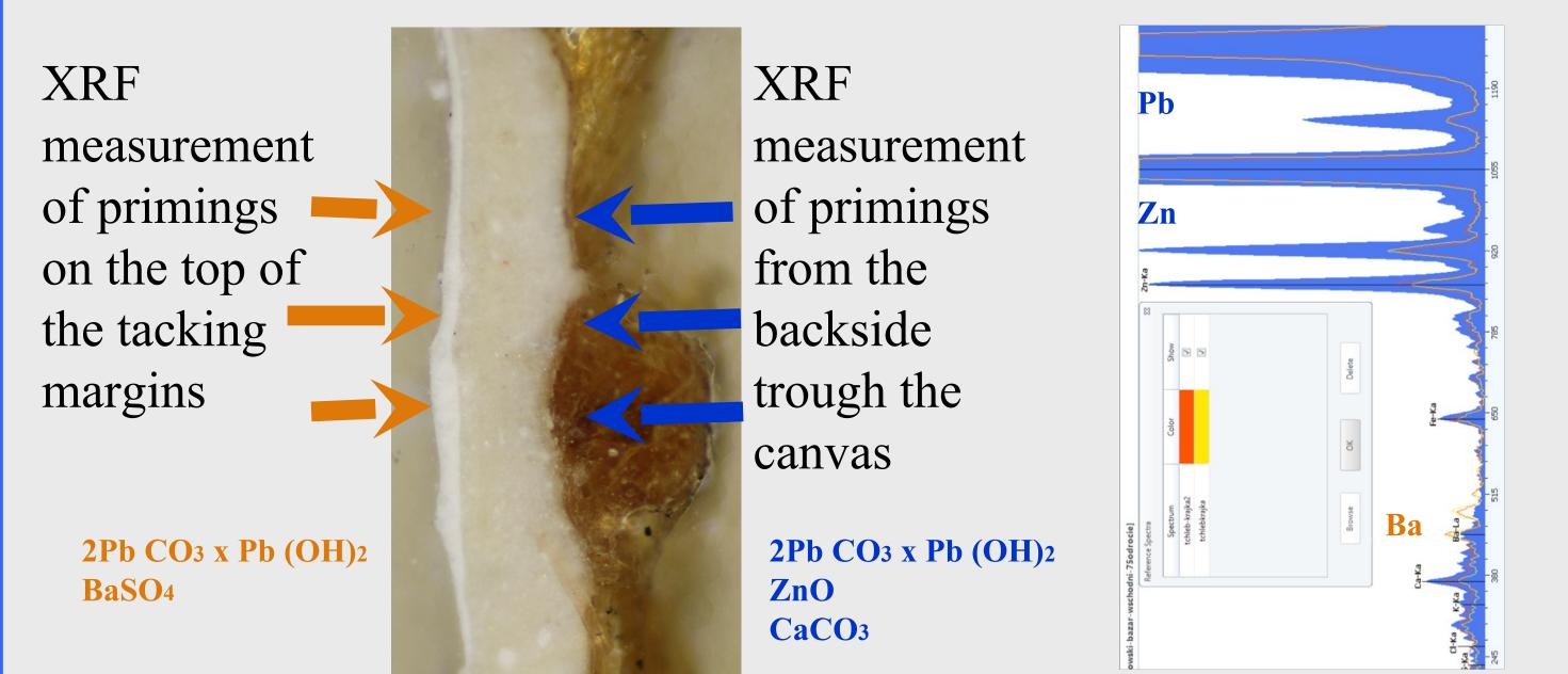
Novel attitude toward the use of XRF and execution of FTIR equipped with movable light trasmiting arm ATR probe enables new non-ivasive approach of the primings research, broadenning its possiblities.
