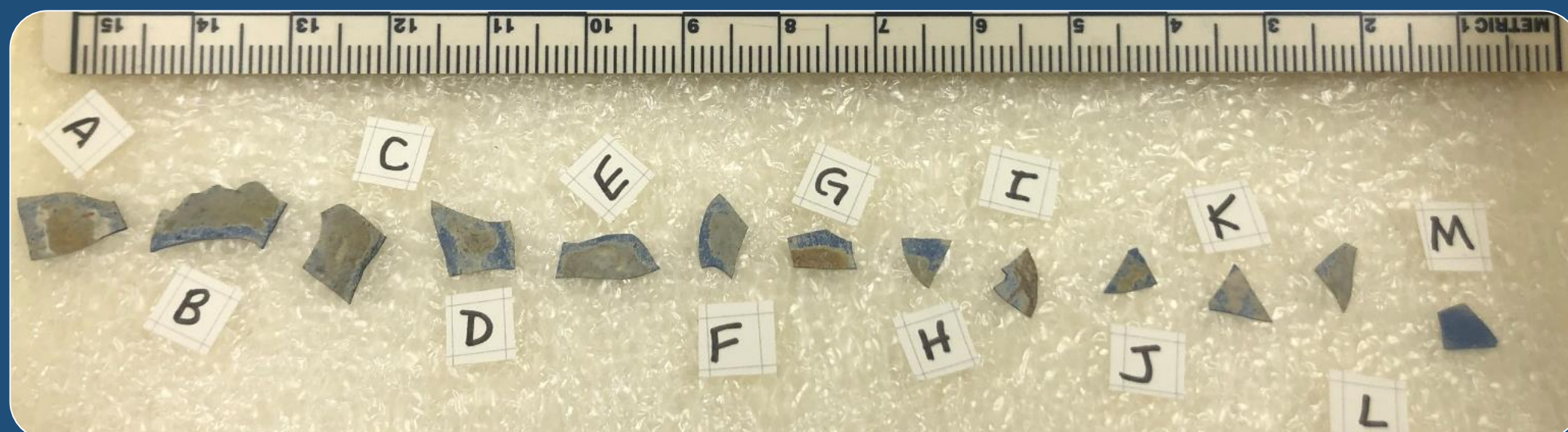
Samples tested; Samples A-F with ammonium citrate, Samples G-L with EDTA, and M as control. BT.
