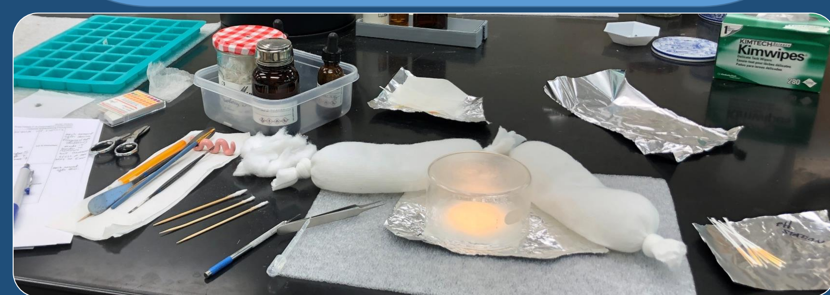
Above, Testing setup under a stereomicroscope with the sample placed under the aluminum foil and a crystallizing dish with clean cotton swabs and pH strips prepared.
