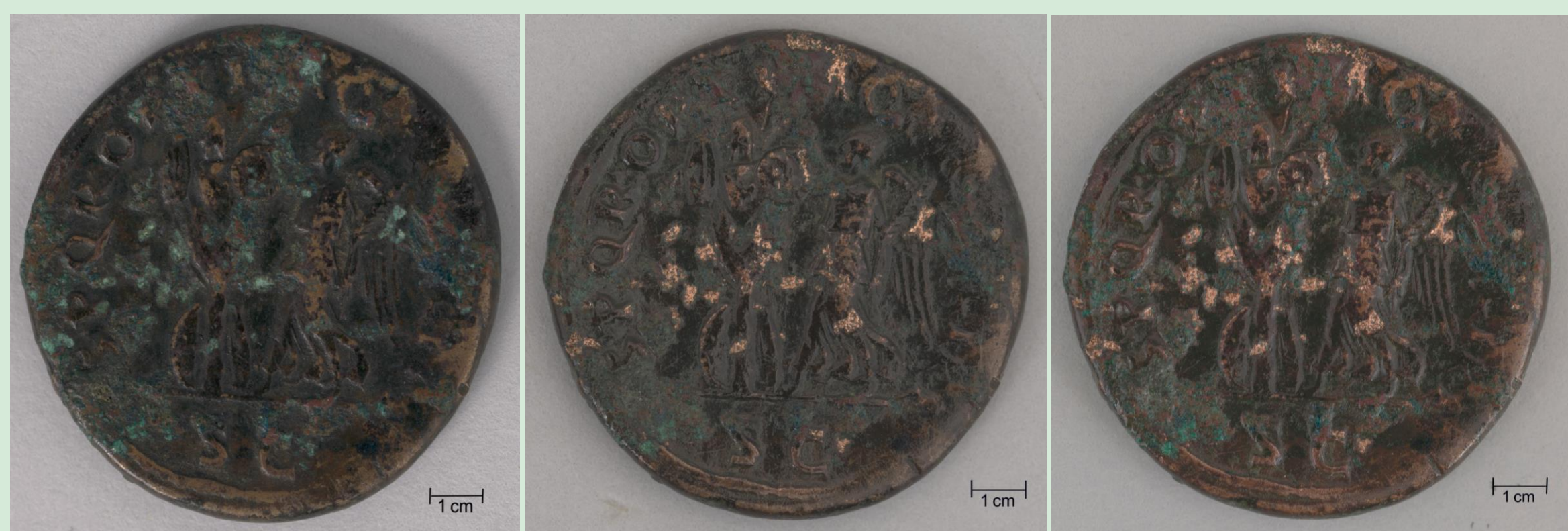
Figure 1. VMFA # 81.135 Roman 1st c. CE, copper with traces of lead, arsenic, and iron, before treatment (left), after treatment (center), after exposure to high humidity (right)
