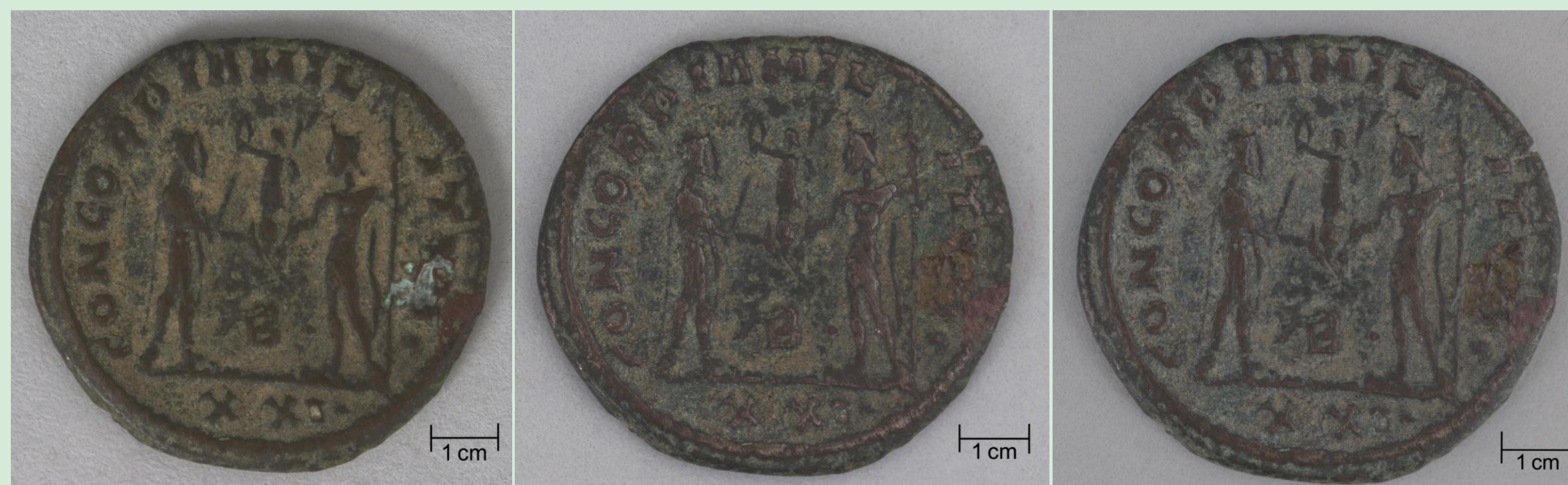
Figure 2. VMFA # 88.72 Roman 3-4th c. CE bronze with traces of silver, lead, and arsenic, before treatment (left), after treatment (center), after exposure to high humidity (right)
