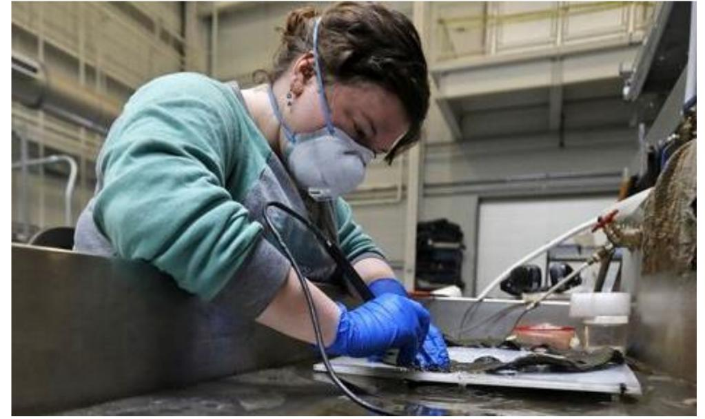
Figure 3. Laurie King surface cleaning rubber gasket using with Parkell TurboSENSOR™ Ultrasonic Scaler. Image Credit: Jonathon Gruenke of Daily Press
