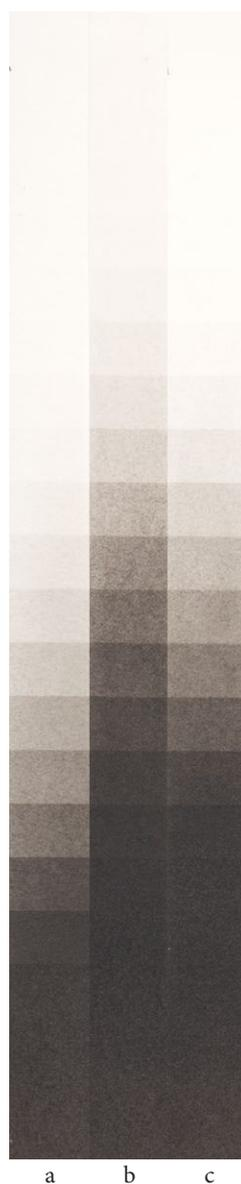
Figure 2. Platinum step-tablets made by the Photograph Conservation Department, National Gallery of Art. (a) Conventionally developed. (b) Glycerine-developed. (c) Glycerine-developed with a dichromate additive to boost contrast. The glycerine-development process extends the range and yields a slightly more smooth-grained image.
