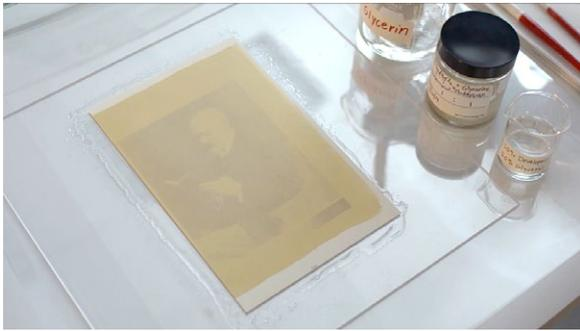
4b. Placing the unexposed print and coating it with glycerine.
