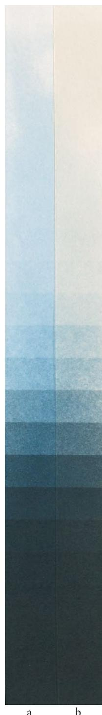
Figure 5. Platinum step-tablets made by the Photograph Conservation Department, National Gallery of Art. (a) Unaged print. (b) Aged print. These step-tablets show the effects of adding ferricyanide to the platinum developer. The blue tone is commonly referred to as “moonlight effects.” Note the loss of blue in the aged sample (b).
