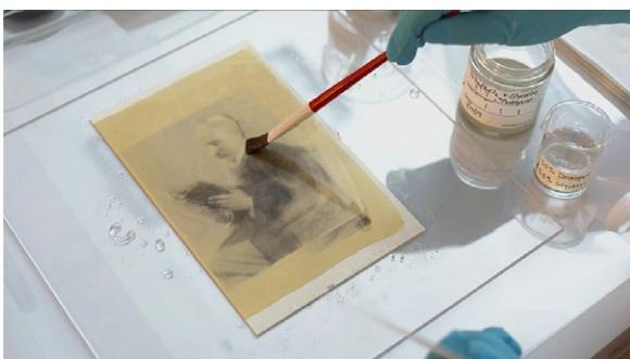
4e. Developing the image using locally applied developer.
