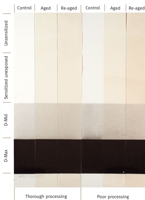
Figure 1. Platinum print step-tablets prepared at the National Gallery of Art using ferric oxalate and potassium tetrachloroplatinate. The prints were either thoroughly processed (left set) or poorly processed. After repeated cycles of accelerated aging, both sets show discoloration, with the poorly processed prints yielding more dramatic staining.
