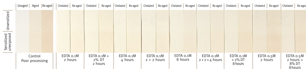
Figure 2. Poorly processed platinum print step-tablets subjected to EDTA chelation. The images are cropped to focus on the sensitizer stain. The poorly processed print was artificially aged and subjected to a range of chelating variables, then finally re-aged. The samples above, grouped in pairs, show the print after chelation and after being re-aged.
