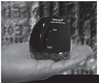
12 - 140x magnification < 2 micron resolution USB powered
